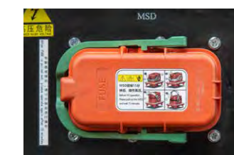
The MSD maintenance switch
