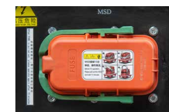
The MSD maintenance switch
